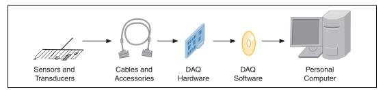
Figure 2-1. Components of a Typical DAQ System
